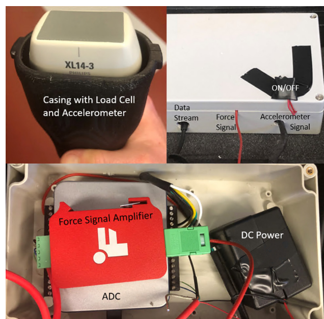
▲ Figure 1: Top left: Custom-made force-coupled ultrasound casing for Philips XL14-3 xMATRIX ultrasound probe. Top right: Closed electronics box with force and accelerometer analog inputs from the casing and data streaming to a tablet for data collection and display. Bottom: Electronics box components consisting of the DC power source of two series 9V batteries, the force signal amplifier, and the multi-channel analog-to-digital converter.
